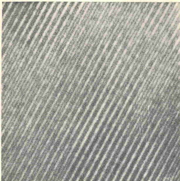
Fig. 3. Electron micrograph of undecomposed \gamma -FeOOH showing (120) lattice planes of spacing 3,3 Å. Hitachi HU-12A. Magnification 5000000
